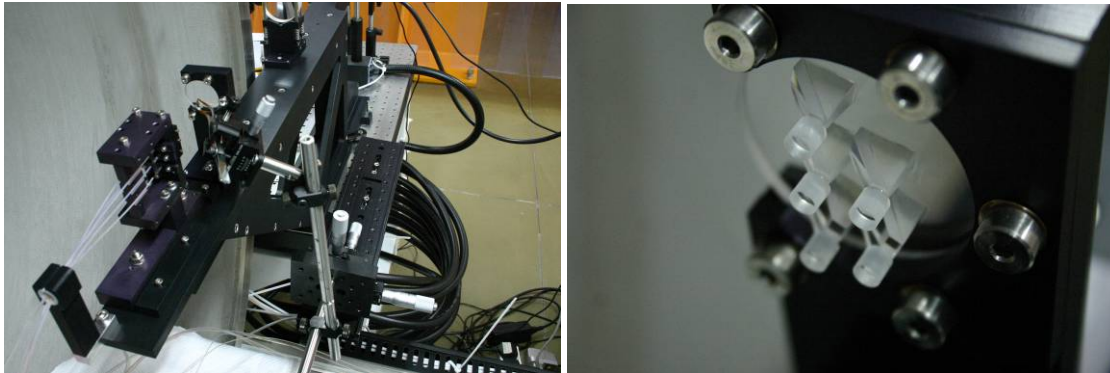
Figure 8 Image slicer manipulation apparatus (left) and close-up of first 5 slicers (right)
