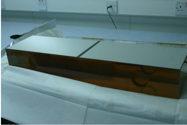
Figure 2 The échelle grating during delivery inspection
