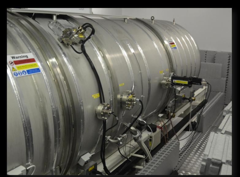
The Fibre Instrument Feed (above left) at prime focus couples the HRS fibres to the telescope. The brass ferrules are attached to translation stages for mode pair selection (vertical) and object/sky fibre separation (horizontal) adjustment. The HRS is enclosed in a steel vacuum tank (above right), which is bricked inside a Styrostone enclosure for insulation against the destabilizing effects of temperature and air pressure variations. The room temperature is also controlled within 0.5°C.
