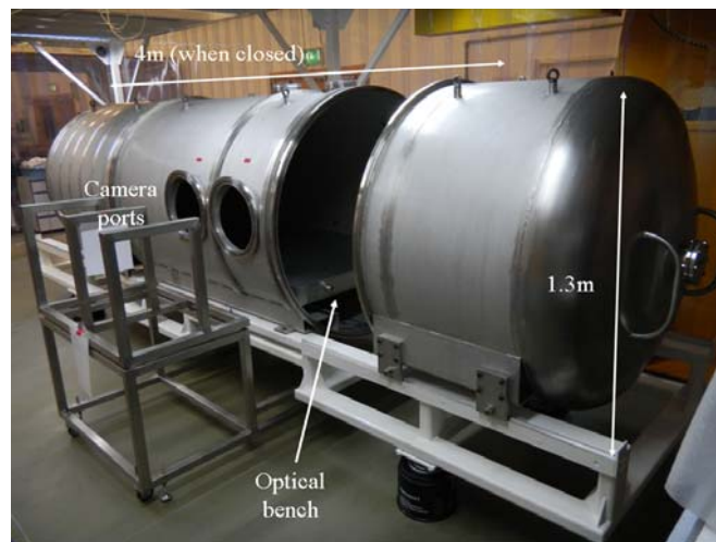
Figure 9. SALT HRS Vacuum Tank, 4 m long and 1.3 m in diameter. The rails upon which it sits allow the tank sections to be separated.
